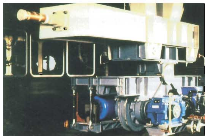
PMO.7 brake drum coupling and a PMO.7 spacer coupling on a John Henderson coal charging car at BSC Dawes Lane.
